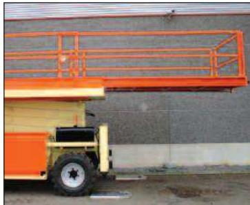
LIFTLUX machines are delivered with standard 4 wheel drive, differential lock and wide foam filled tyres for improved rough terrain capability.
