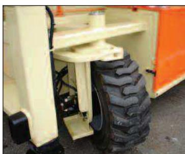
The NIVOLUX outrigger device allows a +/- 0.1° automatic self-leveling of the unit on slopes and uneven ground, reducing the time taken to position the machine.
